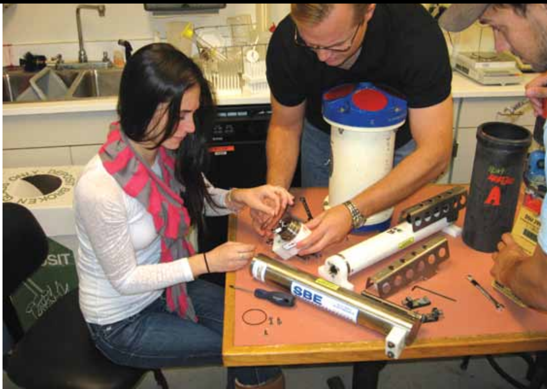
Perri Fine '12 with MSC Manager Shaun Gill and Ryan Knotek '12 in the lab reinstalling o-ring seals that keep instruments water-tight ...
