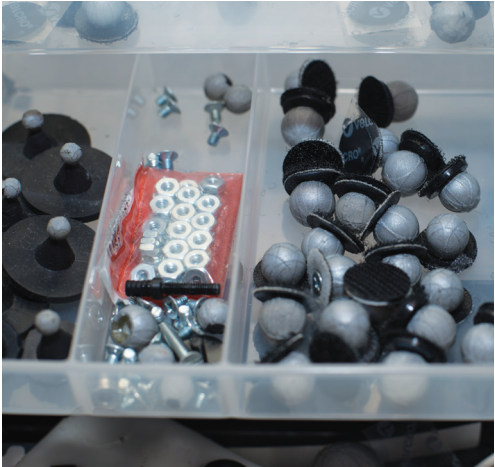
Motion analysis markers used to track motion in 3-D
