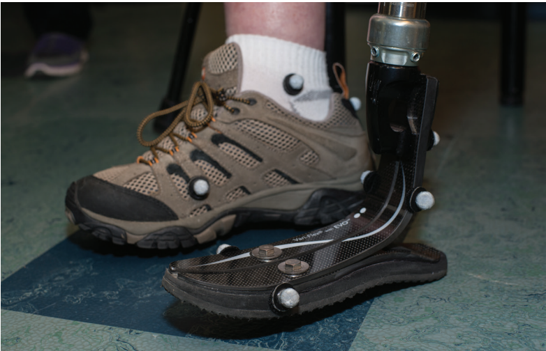
Markers on a prosthetic foot and opposite foot to assess push-off force during walking.
