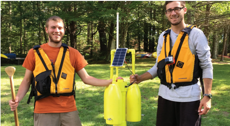
Zach DeLorenzo and Drew Fortin prepare to launch Version 2 of their remote water quality monitoring buoy.
