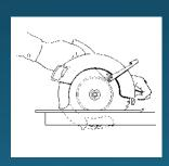
Safety guards must never be removed when a tool is being used.
