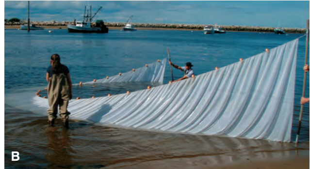
FIGURE 3 (A) Diagram of the multi-mesh gillnets used for sampling the river channel. Image courtesy of Michigan Sea Grant. (B) Beach seine used to sample the river channel along Freddy Beach.
