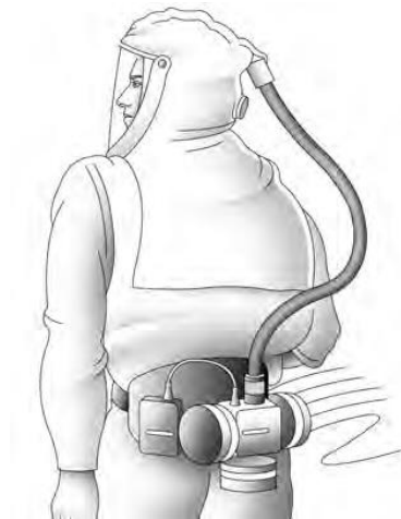
Hood Powered Air-Purifying Respirator (PAPR) APF= 25
