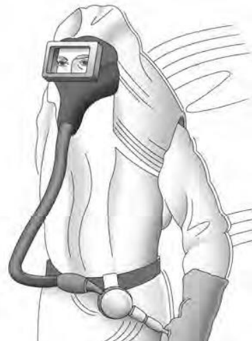
Full Facepiece Abrasive Blasting Continuous Flow APF=1,000 Needs to be fit tested
